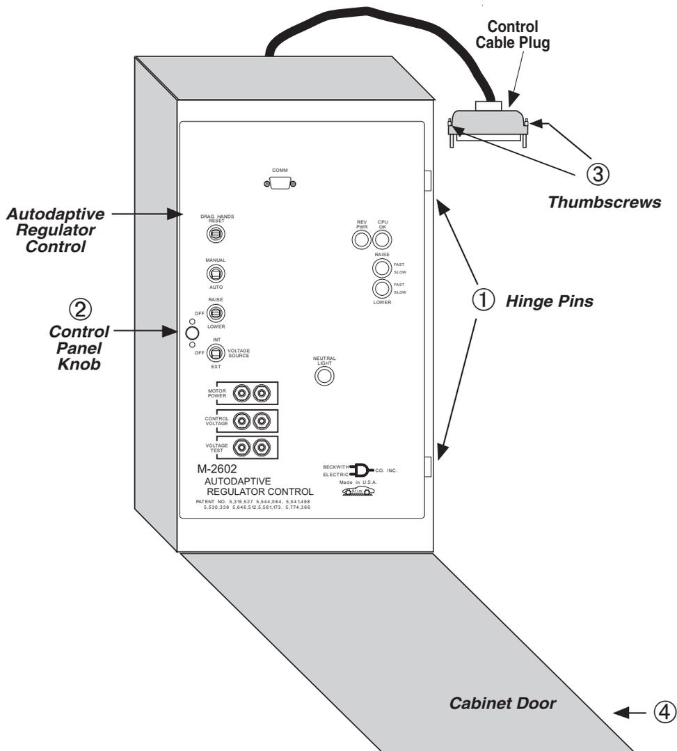
Figure 3-7 M-2602 Autodaptive Regulator Control in Cabinet
