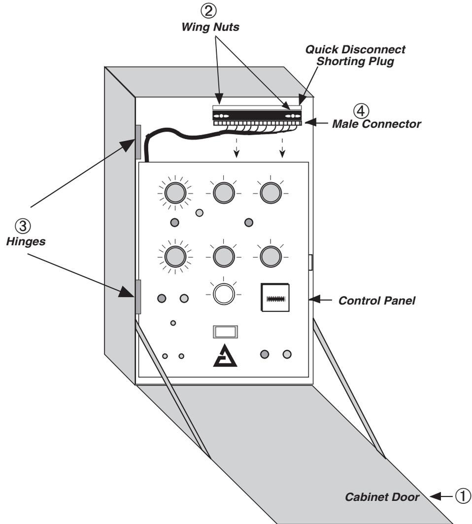
Figure 3-2 Siemens Control in Cabinet
