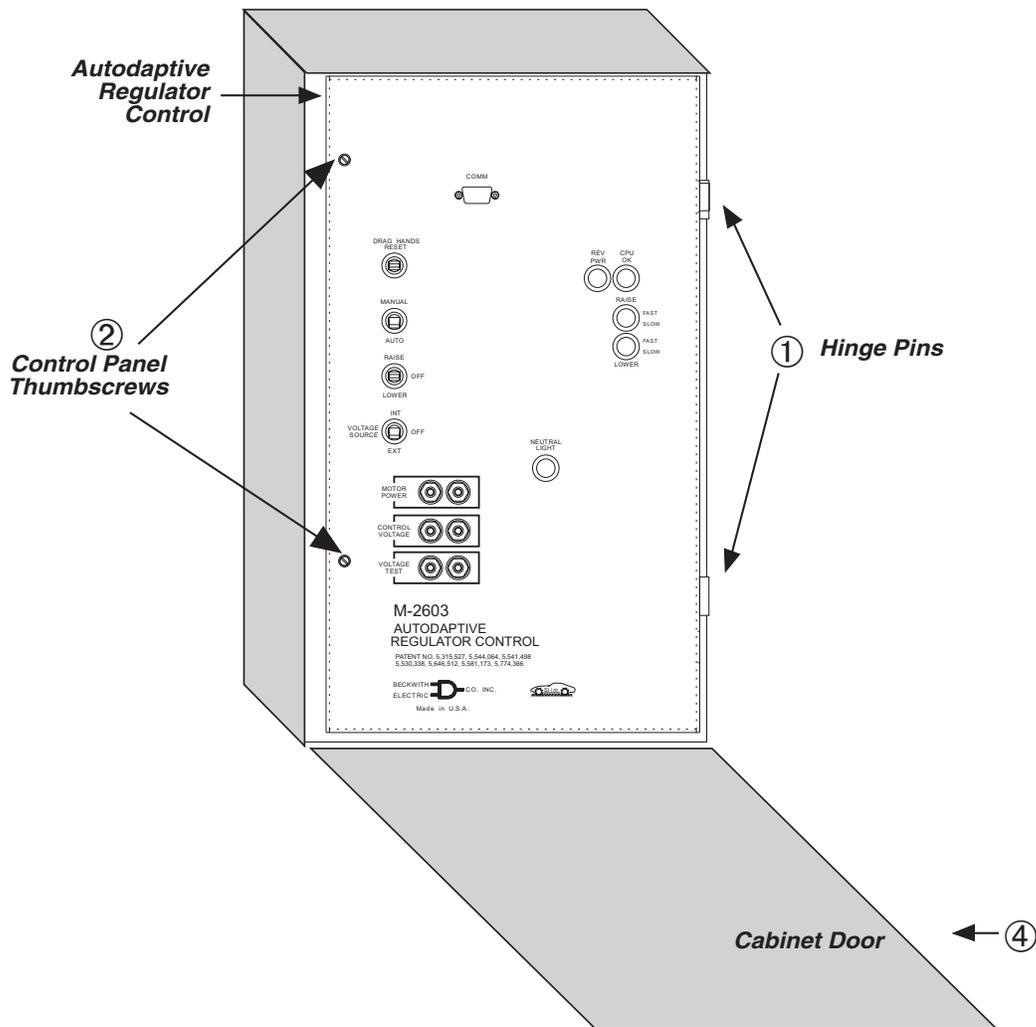
Figure 3-11 M-2603 Autodaptive Regulator Control in Cabinet
