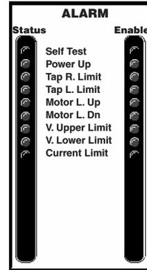
The **Metering Status** screen (see Figure 7-2), contains an array of **Alarm** LEDs that illuminate to indicate a specific Tap Changer Control condition.
