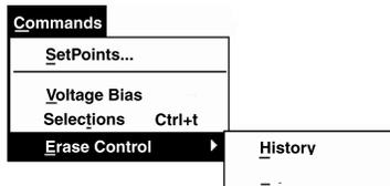
The **Erase Control** submenu allows the user to erase all data for **History** or **Tap Statistics**. This function erases not only the on-board flash in the control, but all downloaded data files stored on your hard drive. To erase current History and Tap Statistics files from the computer only, use the **Erase Data** command from the **File** menu.
