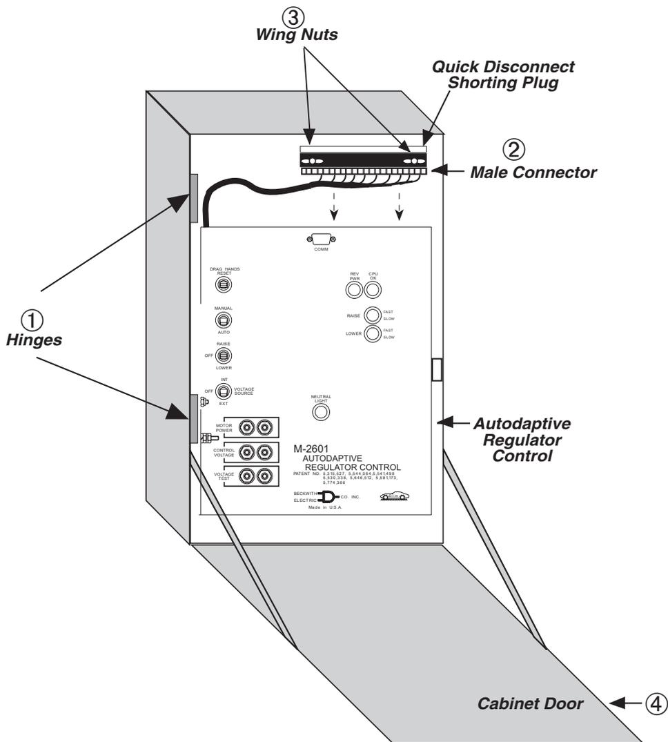
Figure 3-3 M-2601 Adaptive Regulator Control in Cabinet
