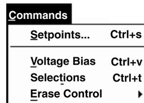
The Commands menu provides three commands (**Setpoints**, **Voltage Bias**, and **Selections**) and one submenu (**Erase Control**) to allow the user select the necessary control functions. Please note that **Voltage Bias** is currently unavailable and will appear greyed-out in display.
