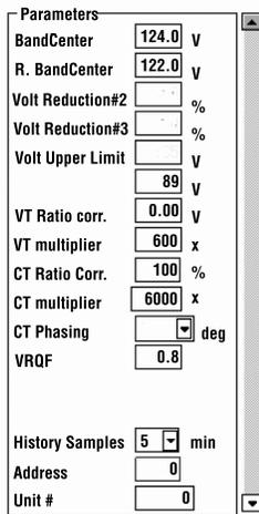
Forward power **Bandcenter** is adjustable from 90.0 V to 135.0 V in 0.1 increments with a factory setting of 120 V.
