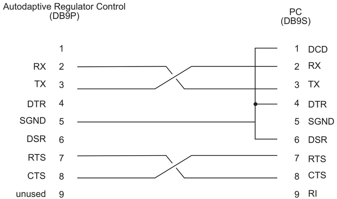
Figure A-1 Null-Modem Cable, 9 pin to 9 pin
