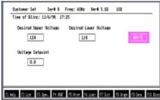
Figure 5 "Voltage Limits" Screen
