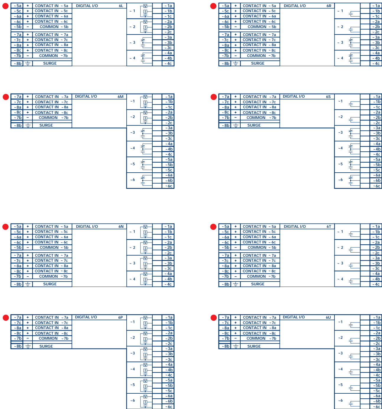
Figure 3-12: DIGITAL I/O MODULE WIRING (SHEET 2 OF 2)
