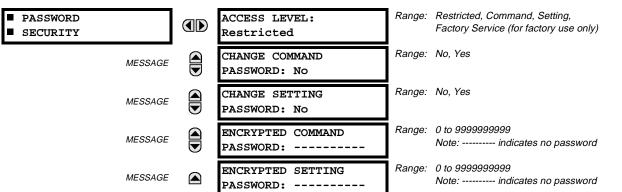
The L90 provides two user levels of password security: Command and Setting. Operations under password supervision are as follows:
