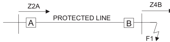
Figure 2–10: ZONE 4 FAULT EXAMPLE
