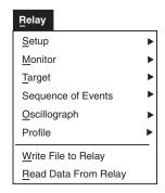
The **Relay** menu provides access to the windows used to set, monitor, or interrogate the relay. Six submenus are provided: Setup, Monitor, Target, Sequence of Events, Oscillograph and Profile as well as two commands, Write File to Relay, and Read Data From Relay.
