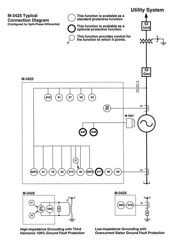
Figure 2-2 Alternative One-Line Functional Diagram
