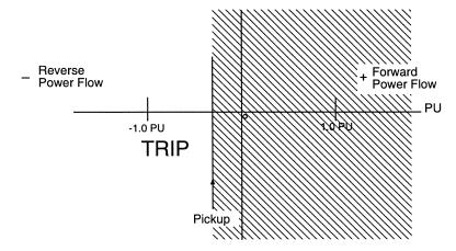
Figure 2-9 Tripping on Low Forward Power in Negative Direction (Toward Generator)
