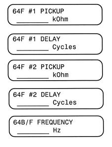
To minimize measurement errors, the 64B/F frequency should be set according to the amount of capacitance across the field winding and the ground. Table 2-23, above, has typical settings of the frequency for capacitance, ranging from 1  $\mu$ F to 10  $\mu$ F.
