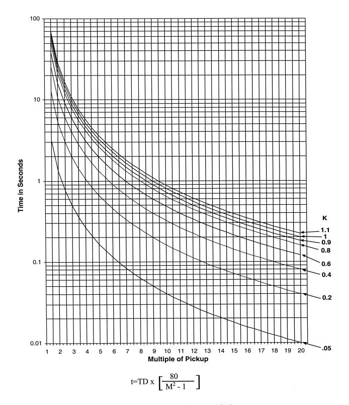
Figure D-11 IEC Curve #3 Extremely Inverse
