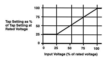
Figure 2-14 Voltage Restraint (51VR) Characteristic
