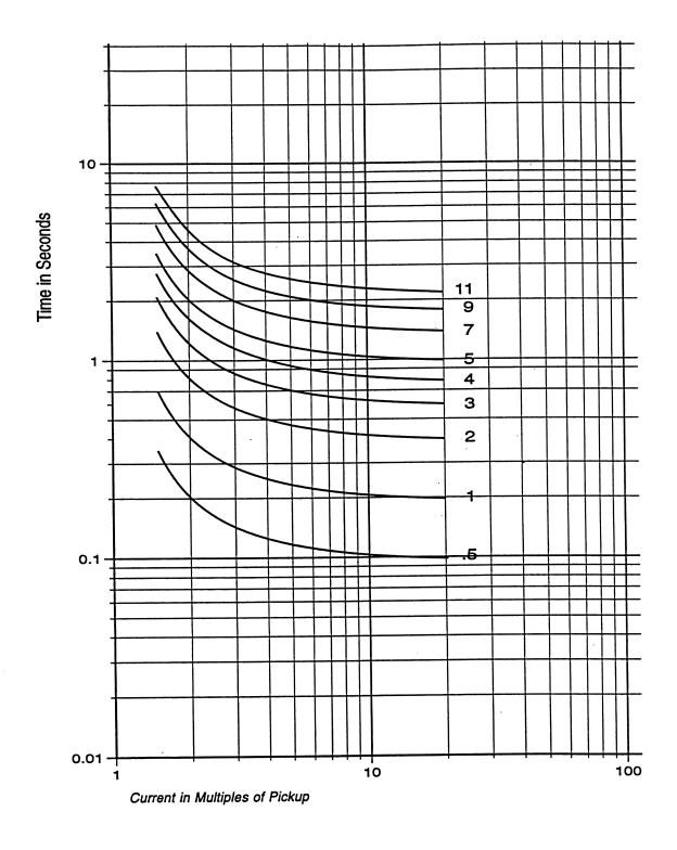
Figure D-5 Definite Time Overcurrent Curve
