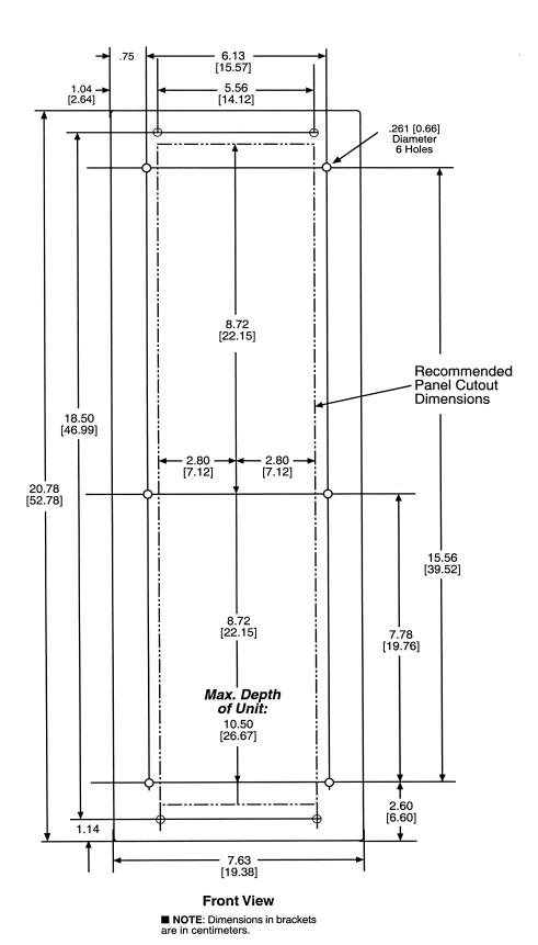
Figure 5-4 (H3) Mounting Dimensions for GE L-2 Cabinet
