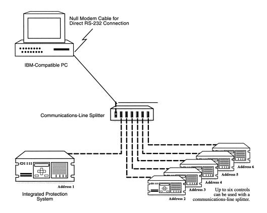
Figure 4-1 Multiple Systems Addressing Using Communications-Line Splitter
