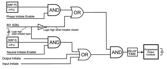
Figure 2-12 Breaker Failure Logic Diagram
