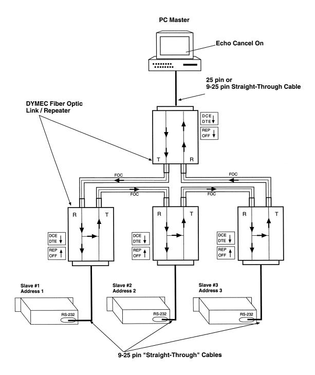
Figure B-2 RS-232 Fiber Optic Network
