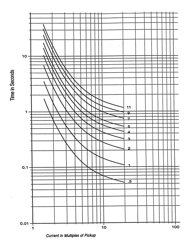
Figure D-7 Very Inverse Time Overcurrent Curve
