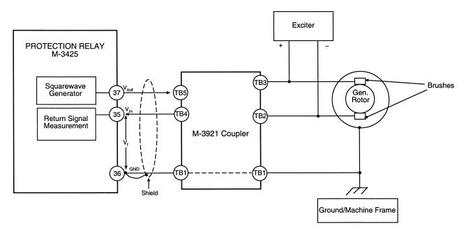
Figure 2-16 M-3921 Field Ground Coupler
