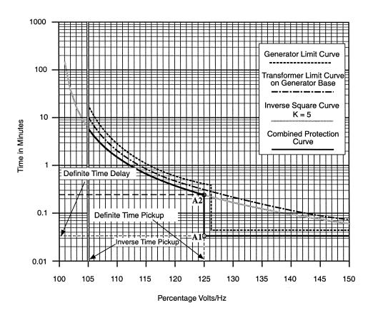
Figure 2-6 Example of Capability and Protection Curves (24)
