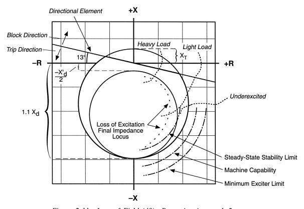
Figure 2-11 Loss of Field (40)—Protective Approach 2
