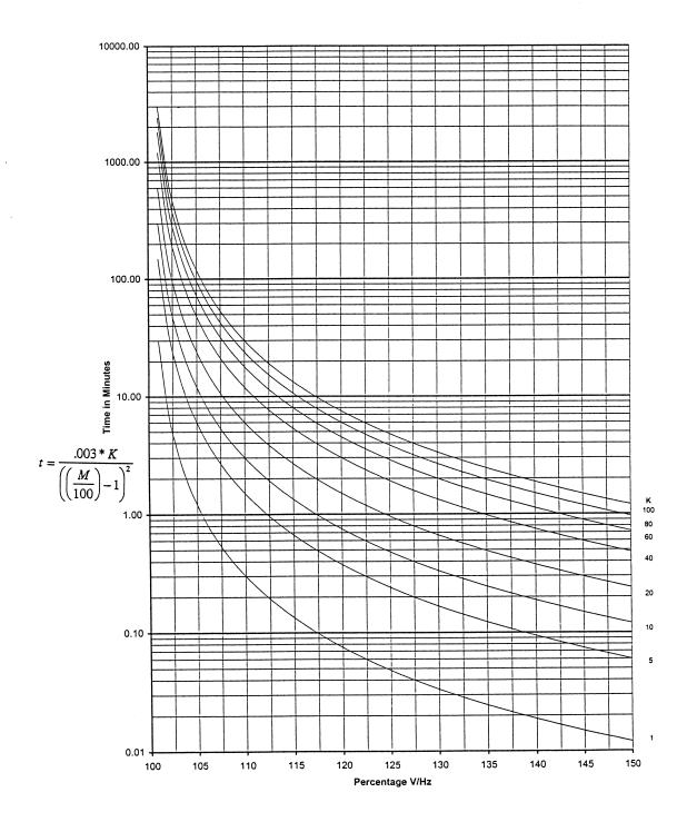
Figure D-1 Volts/Hz (24) Inverse Curve Family #1 (Inverse Square)
