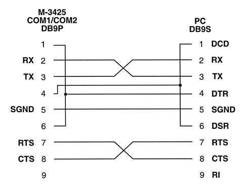
Figure B-1 Null Modem Cable: M-0423
