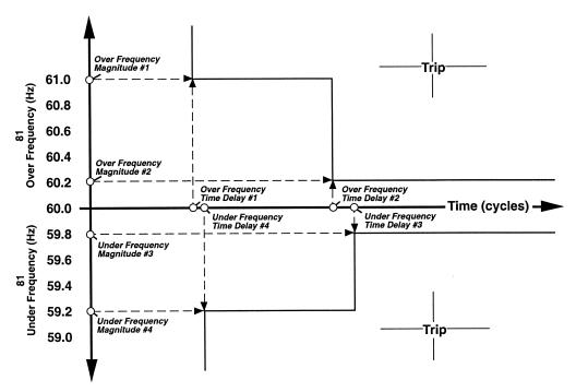
Figure 2-19 Example of Frequency (81) Trip Characteristics
