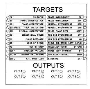
Figure 6-7 M-3925 Target Module Panel
