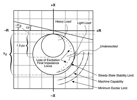
Figure 2-10 Loss of Field (40)—Protective Approach 1
