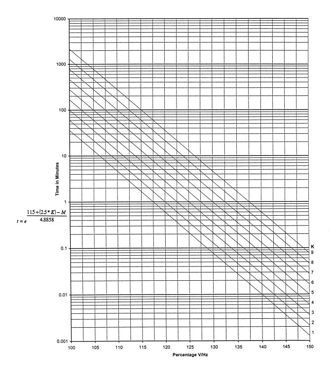
Figure D-2 Volts/Hz (24) Inverse Family Curve #2
