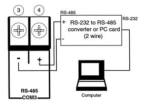
Figure 6-10 RS-485 2-Wire Testing
