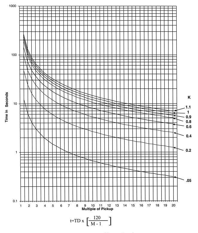
Figure D-12 IEC Curve #4 Long-Time Inverse
