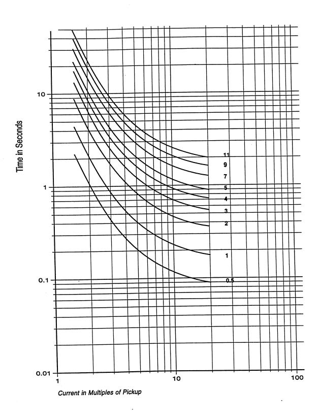
Figure D-6 Inverse Time Overcurrent Curve
