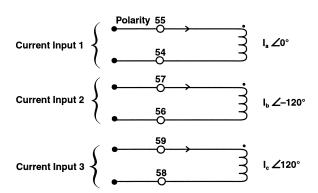
Figure 6-3 Current Inputs: Configuration C1
