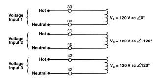
Figure 6-1 Voltage Inputs: Configuration V1
