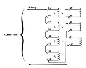
Figure 6-11 Current Input Configuration
