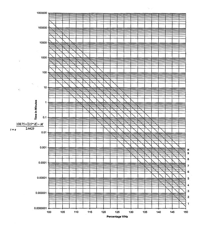
Figure D-4 Volts/Hz (24IT) Inverse Curve Family #4
