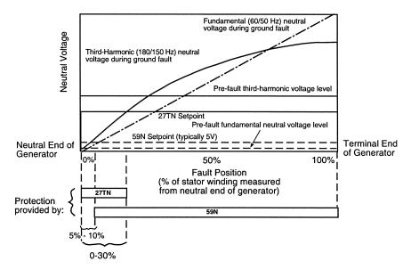
Figure 2-7 Third Harmonic Undervoltage (27TN) Protection Characteristics
