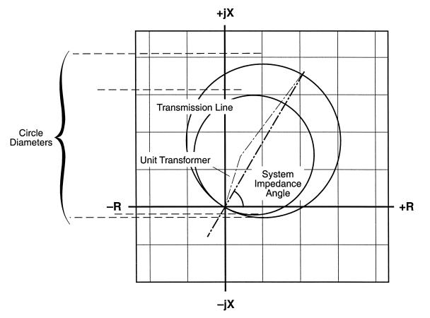
Figure 2-5 Phase Distance (21) Function Applied for System Backup
