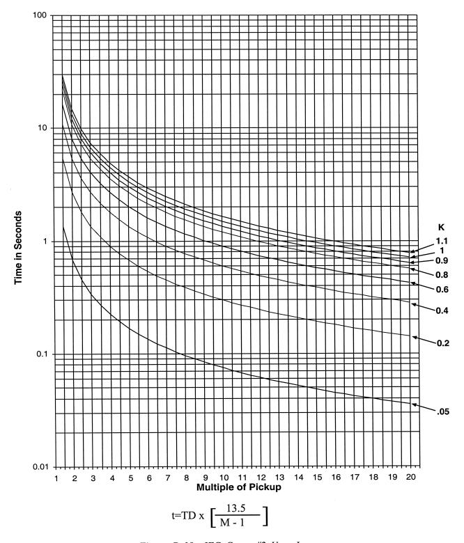
Figure D-10 IEC Curve #2 Very Inverse
