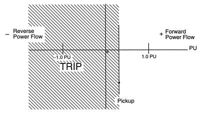
Figure 2-8 Tripping on Low Forward Power in Positive Direction (Toward System)
