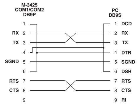
Figure B-1 Cable Null Modem: M-0423
