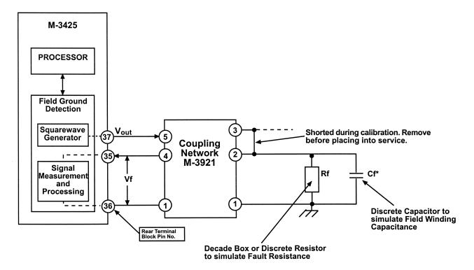
\* If the rotor is NOT connected, the value of Cf should approximate the rotor capacitance. If the rotor is connected Cf is NOT required.
