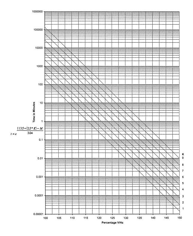
Figure D-3 Volts/Hz (24IT) Inverse Curve Family #3
