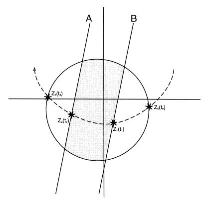
Figure 2-18 Out-of-Step Relay Characteristics
