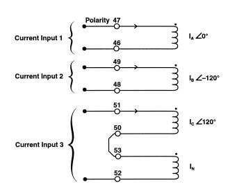
Figure 6-4 Current Inputs: Configuration C2
