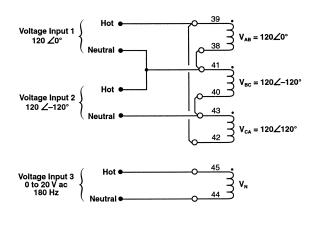
Figure 6-2 Voltage Inputs: Configuration V2
