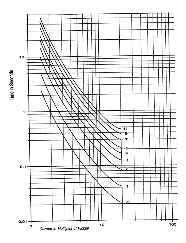
Figure D-8 Extremely Inverse Time Overcurrent Curve
