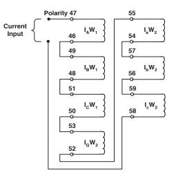
Figure 6-8 Current Calibration Configuration
