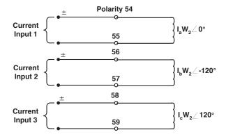
Figure 6-12 Current Inputs, Configuration C2
