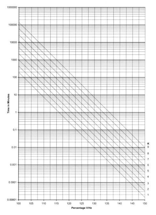
Figure D-3 Volts/Hz (24IT) Inverse Time Curve Family #3
