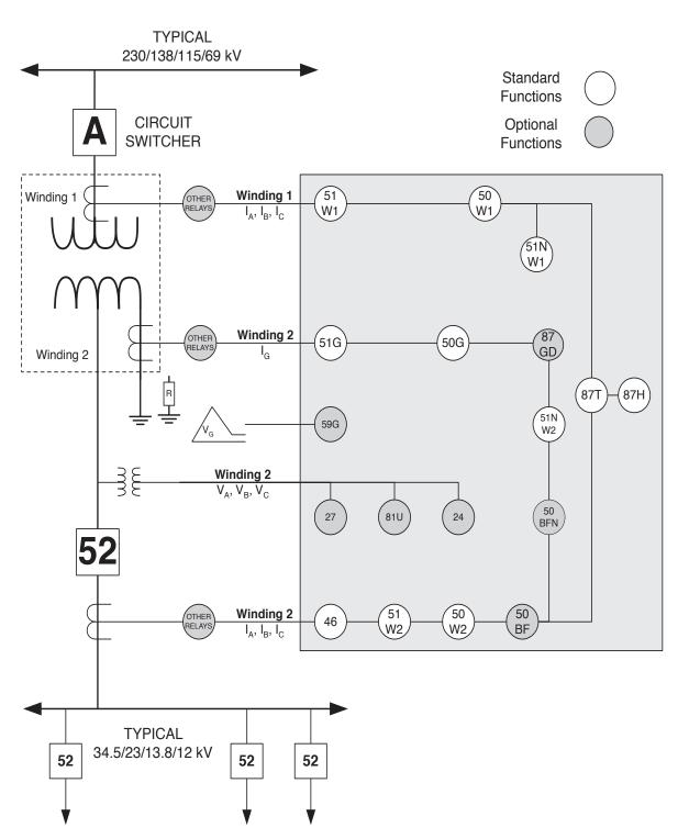
Figure 2-1 One-Line Functional Diagram
