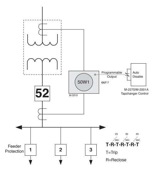
Figure 2-13 LTC Blocking Scheme During Faults
