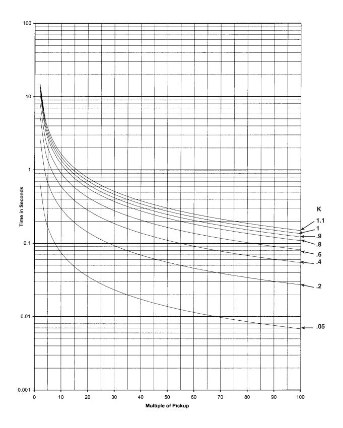
Figure D-10 IEC Curve – Very Inverse
