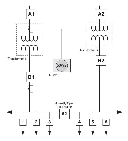
Figure 2-11 Two Bank Load Shedding Scheme
