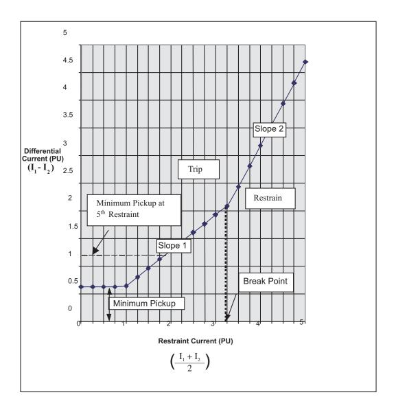
Figure 2-5 87T Programmable Dual Slope Percentage Characteristics
