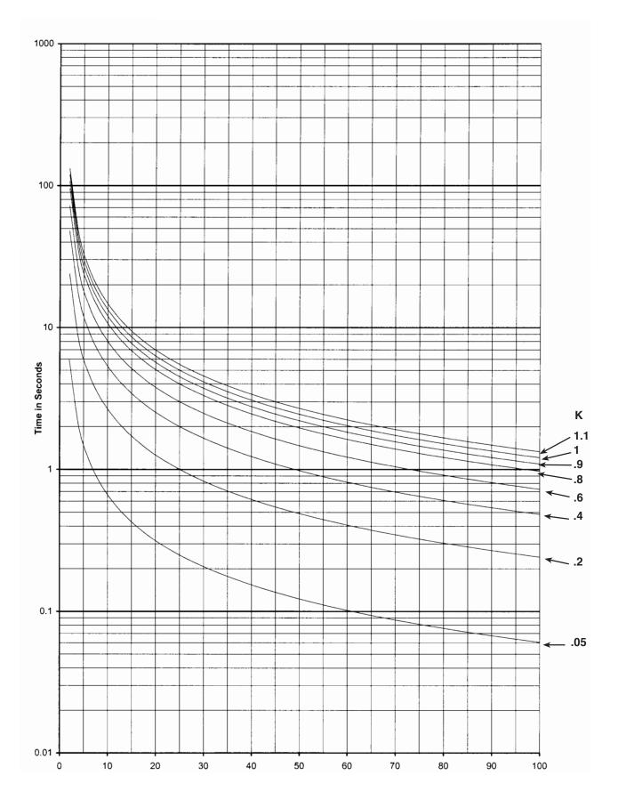
Figure D-12 IEC Curve – Long-Time Inverse
