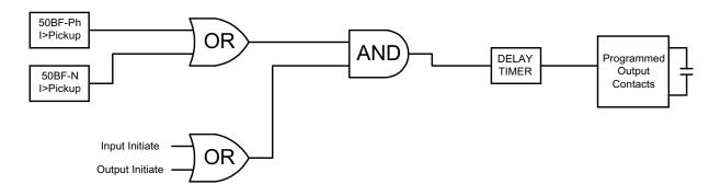
Figure 2-4 Breaker Failure Logic Diagram
