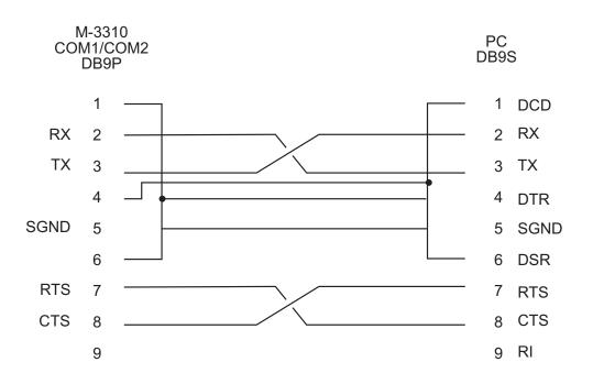
Figure B-1 Null Modem Cable for M-3310
