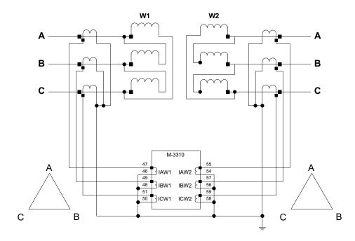
Type 11: Delta-AB/Delta-AB Power Transformer with Wye/Wye CT Connection
