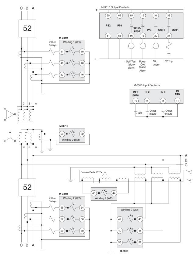
Figure 5-6 Three-Line Connection Diagram with Broken Delta-connected VTs
