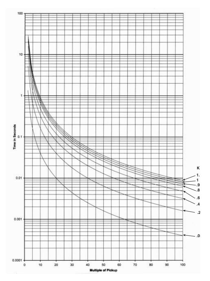
Figure D-11 IEC Curve – Extremely Inverse
