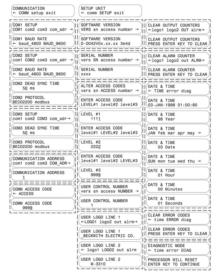
Figure 3-5 Sample of Communication Data & Unit Setup Record
