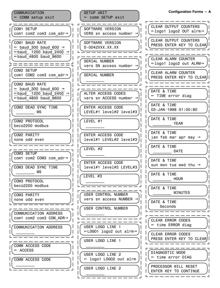
Figure A-2 Communication Data & Unit Setup (Page 2 of 2)
