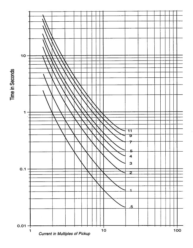
Figure D-8 Extremely Inverse Time Overcurrent Curve
