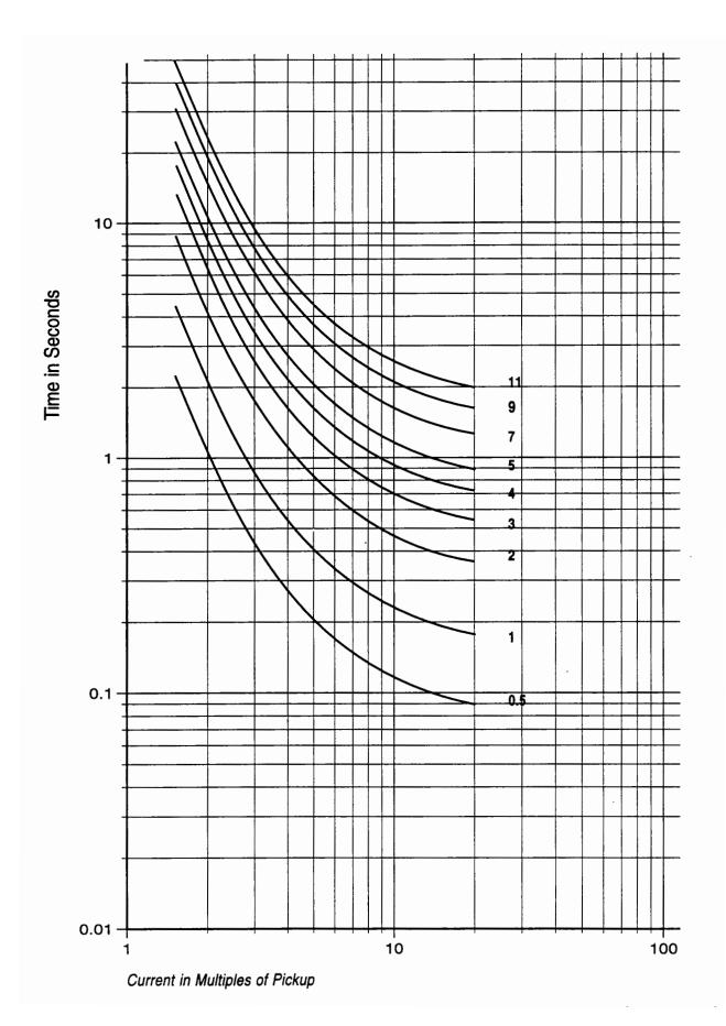
Figure D-6 Inverse Time Overcurrent Curve
