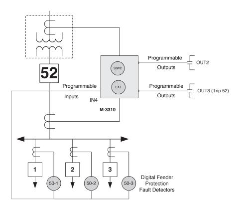
Figure 2-7 Bus Fault Protection Scheme
