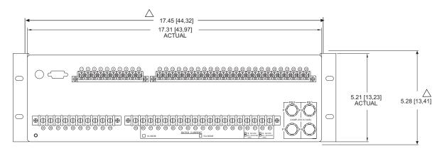
REAR VIEW A RECOMMENDED CUTOUT WHEN RELAY IS NOT USED AS STANDARD RACK MOUNT
