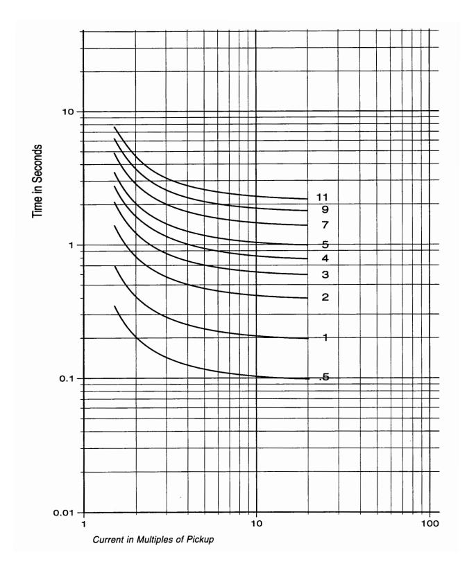
Figure D-5 Definite Time Overcurrent Curve
