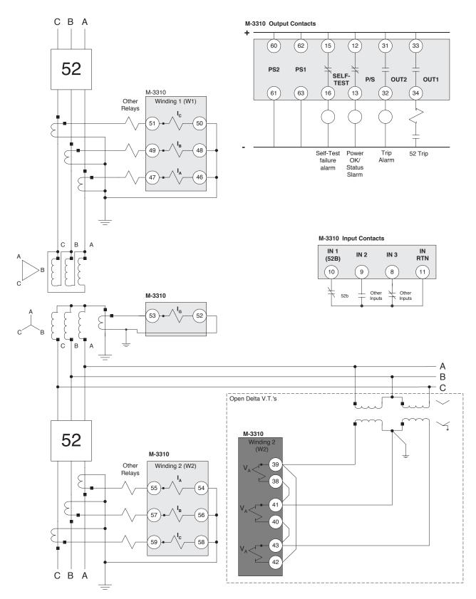
Figure 5-7 Three-Line Connection Diagram with Open Delta-connected VTs
