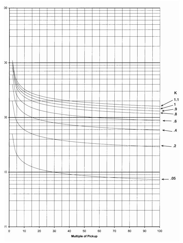
Figure D-9 IEC Curve – Inverse
