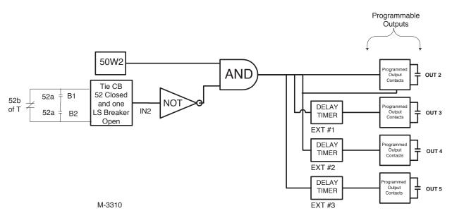
Figure 2-12 Load Shedding Logic
