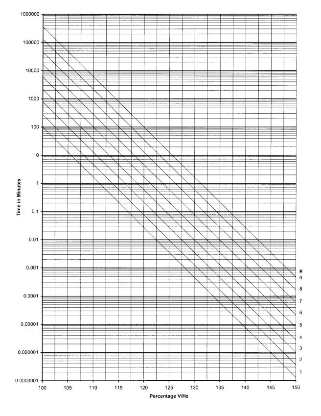
Figure D-4 Volts/Hz (24IT) Inverse Curve Family #4
