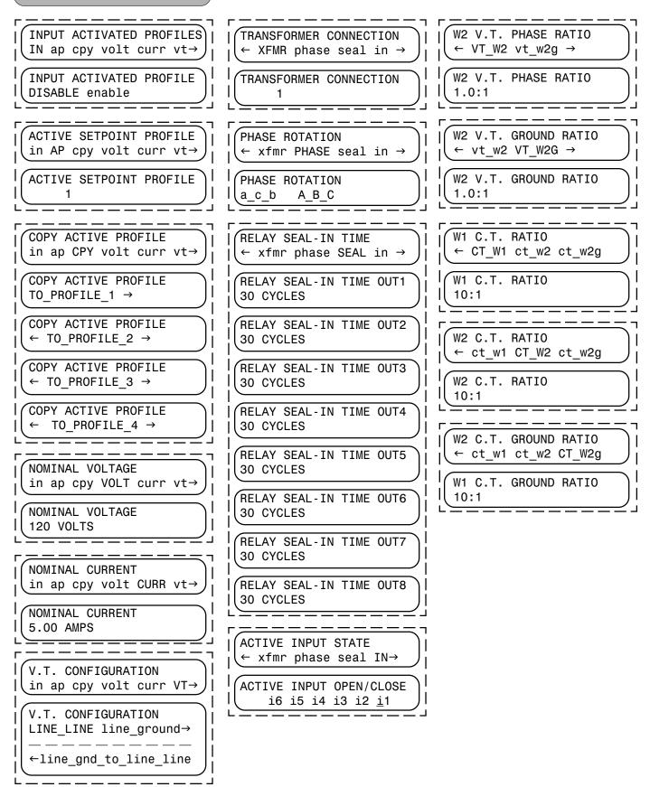
A-12 Figure A-2 Communication Data & Unit Setup – As Shipped (Page 1 of 2)
