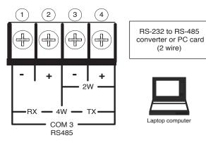
Figure 6-5 RS-485 2-Wire Testing
