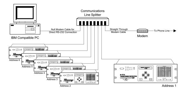
Figure 4-2 Multiple Systems Addressing Using Communications-Line Splitter
