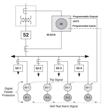
Figure 2-9 Digital Feeder Relay Backup Scheme
