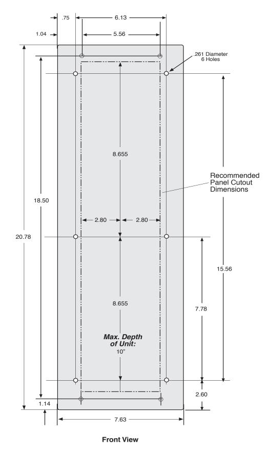
Figure 5-4 (H3) Mounting Dimensions for GE L-2 Cabinet
