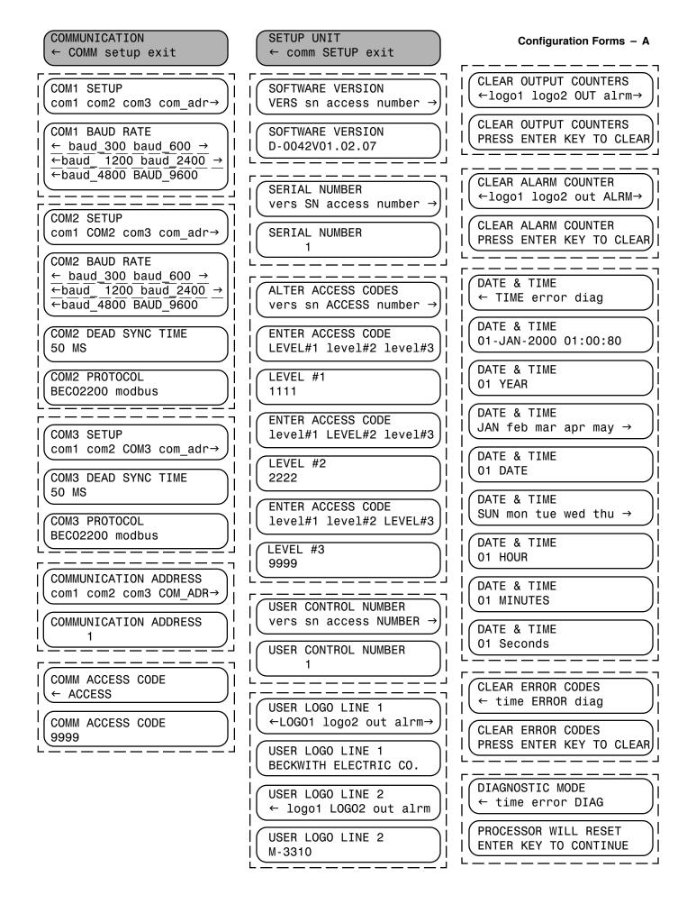
Figure A-2 Communication Data & Unit Setup – As Shipped (Page 2 of 2)
