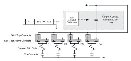
Figure 2-10 Feeder Backup Logic
