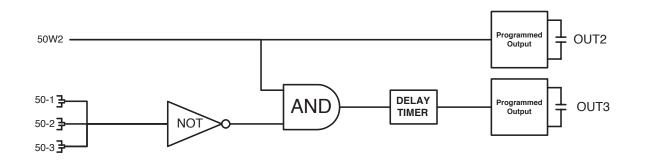
Figure 2-8 Bus Fault Protection Logic
