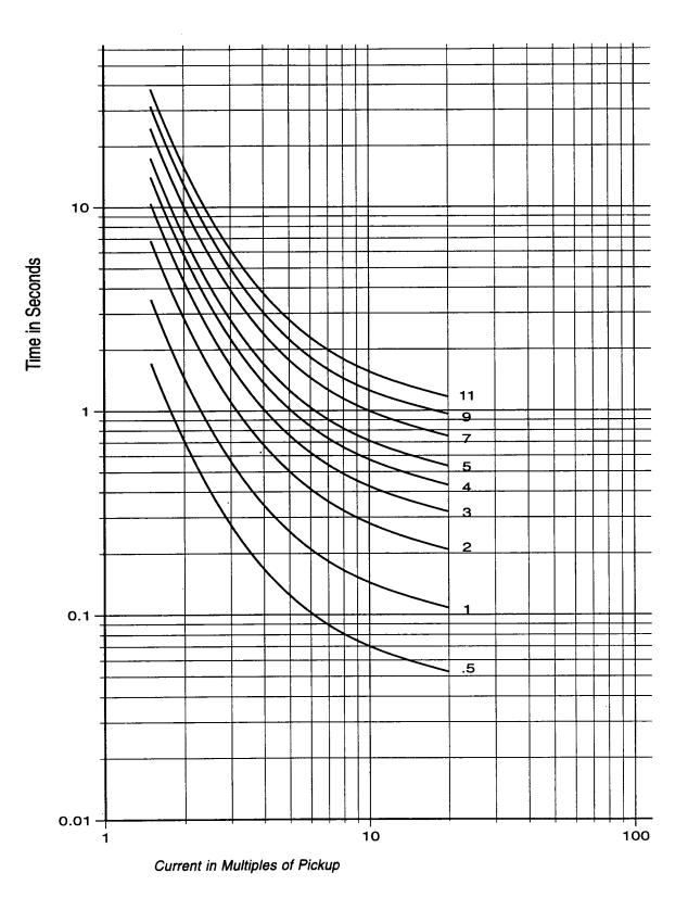
Figure D-7 Very Inverse Time Overcurrent Curve
