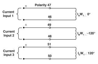
Figure 6-11 Current Inputs, Configuration C1
