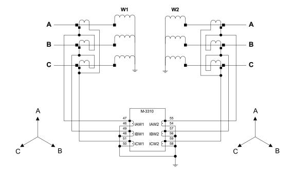
Type 7: Wye/Wye Power Transformer with Delta-AB/Delta-AB CT Connection
