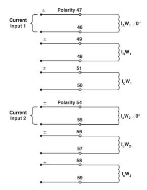
Figure 6-14 Current Inputs, Configuration C4
