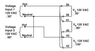
Figure 6-10 Voltage Inputs, Configuration V2
