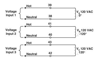
Figure 6-9 Voltage Inputs, Configuration V1
