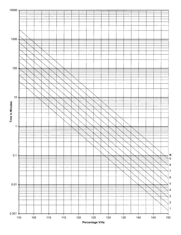
Figure D-2 Volts/Hz (24IT) Inverse Family Curve #2
