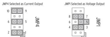
Voltage Output Jumpers Figure 2.5 Current Output Jumpers Figure 2.6
