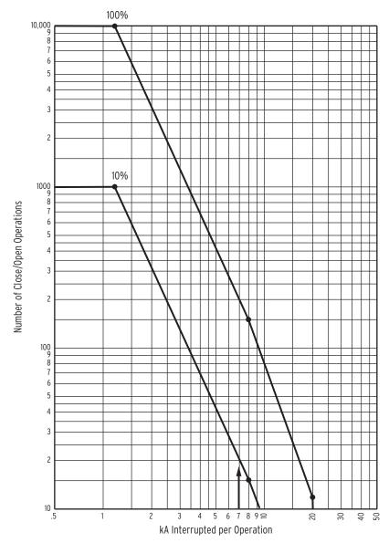
Figure 5.22 Breaker Monitor Accumulates 10 Percent Wear
