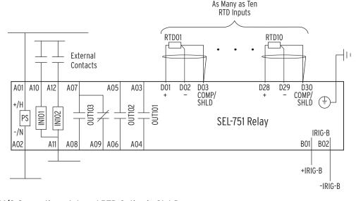
Figure 2.16 Control I/O Connections-Internal RTD Option in Slot D
