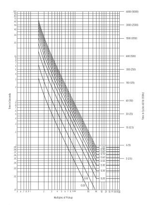
Figure 4.17 IEC Class C Curve (Extremely Inverse): C3
