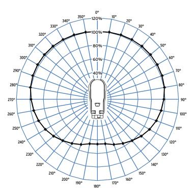
Figure 2.37 Point-Sensor Directivity (0-360° Around the Mounting Plane)
