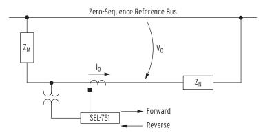
Figure 4.44 Zero-Sequence Impedance Network and Relay Polarity
