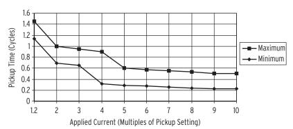
Figure 4.3 Instantaneous Overcurrent Element Pickup Time Curve
