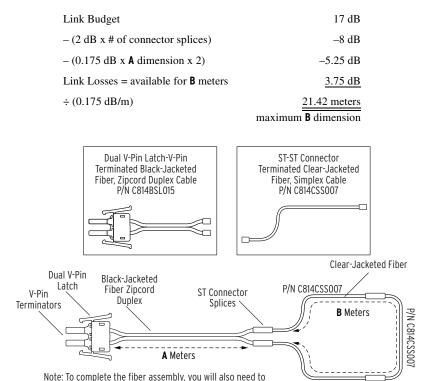
Figure 2.47 Bare-Fiber Sensor Assembly With Two Additional ST Splice Connectors
