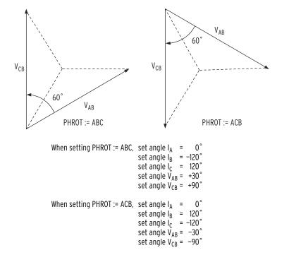
Figure 11.3 Three-Phase Open-Delta AC Connections
