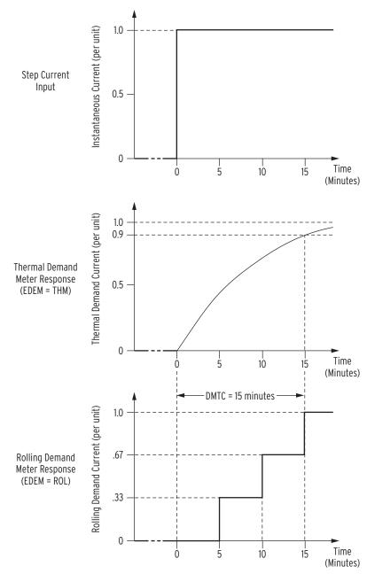
Figure 4.91 Response of Thermal and Rolling Demand Meters to a Step Input (Setting DMTC = 15 minutes)
