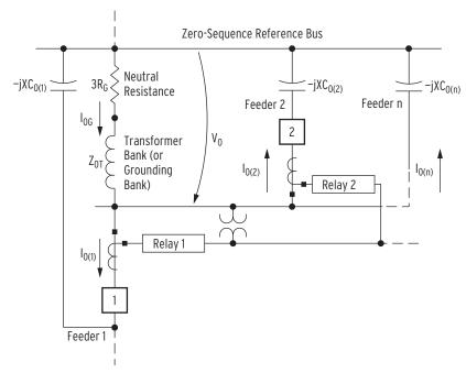
Figure 4.47 Zero-Sequence Impedance Network for Low-Impedance Grounded Distribution System With a Ground Fault on Feeder 1
