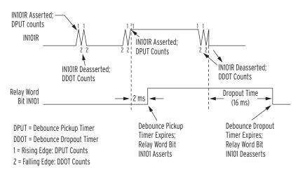
Figure 4.111 Timing Diagram for Debounce Timer Operation When Operating in AC Mode
