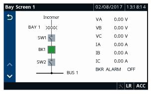
Figure 9.25 Incomer With Step-Down Transformer Bay Control Single-Line Diagram
