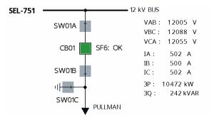
Figure 9.10 Bay Control Single-Line Diagram Schematic
