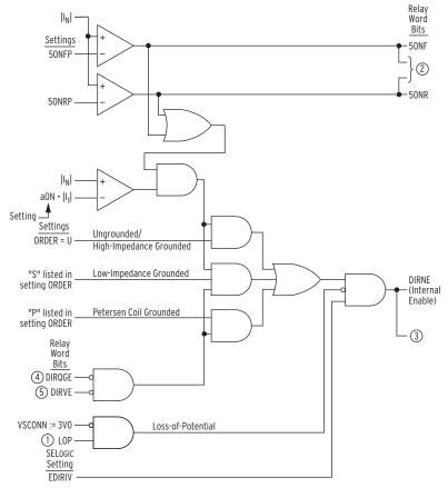
**NOTE:** Residual ground current  $I_G$  is used in place of neutral current  $I_N$  under certain circumstances. See Switch Between  $I_N$  and  $I_G$  for Low-Impedance Grounded and Ungrounded/High-Impedance Grounded Systems on page 4.31.
