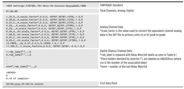
Figure 10.10 Sample COMTRADE .CFG Configuration File Data (Sheet 1 of 2)
