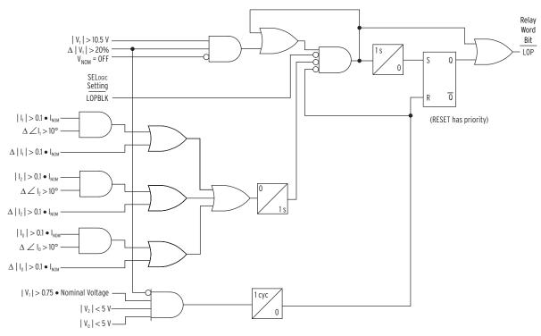
Note:  $I_{\text{NOM}}$  is 1 A or 5 A depending on the part number. I<sub>NOM</sub> is the phase secondary input rating.
