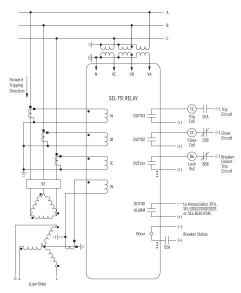
Voltages are necessary for voltage elements, synchronism-check elements, voltage-polarized directional elements, fault location, and metering (e.g., voltage, KW, KVAR). INxxx and OUTxxx indicate user-configurable optional digital inputs and outputs.
