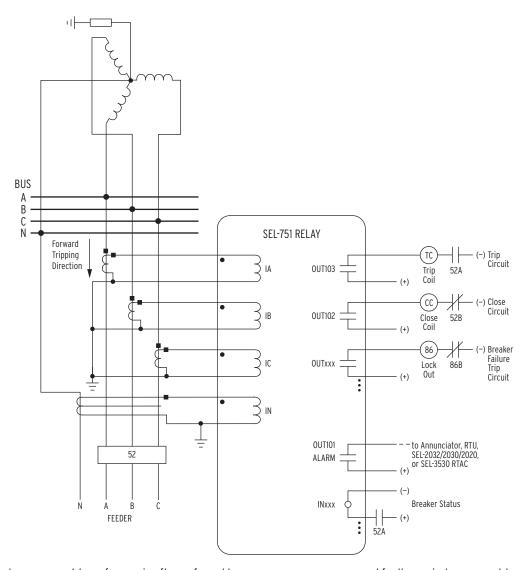
A core-balance current transformer is often referred to as a zero-sequence, ground fault, or window current transformer.
