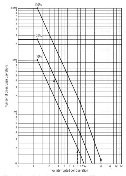
Figure 5.23 Breaker Monitor Accumulates 25 Percent Wear
