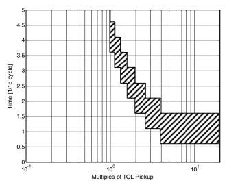
Figure 4.104 TOL Element Inverse Curve Characteristic
