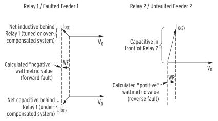
Figure 4.53 Wattmetric Element Operation for Ground Fault on Feeder 1
