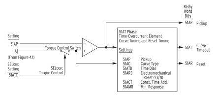
Logic State of 51ATC Controls the Torque Control Switch
