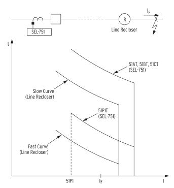
Figure 4.87 Sequence Coordination Between the SEL-751 and a Line Recloser
