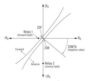
Figure 4.51 ZOMTA Setting Provides Forward/Reverse Ground Fault Discrimination in a Low-Impedance Grounded Distribution System
