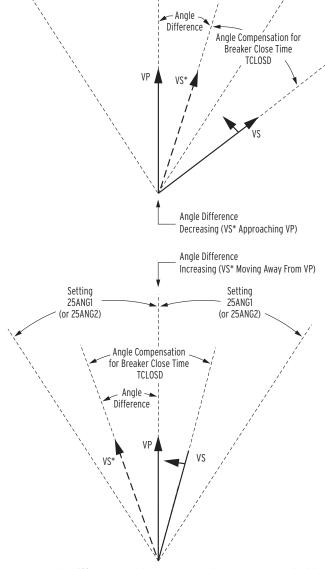
Figure 4.69 Angle Difference Between VP and VS Compensated by Breaker Close Time (fP < fS and VP Shown as Reference in This Example)
