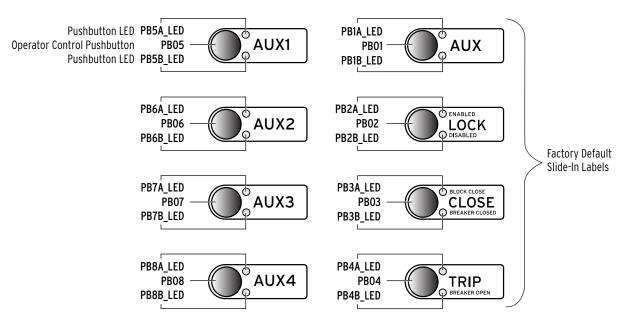
Figure 8.27 Operator Control Pushbuttons and LEDs
