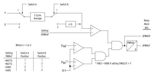
Figure 4.70 Three-Phase Power Elements Logic
