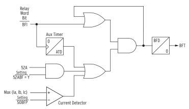
Figure 4.101 Breaker Failure Logic
