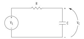
Figure 4.92 Voltage VS Applied to Series RC Circuit
