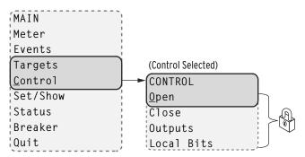
Figure 8.18 MAIN Menu and CONTROL Submenu
