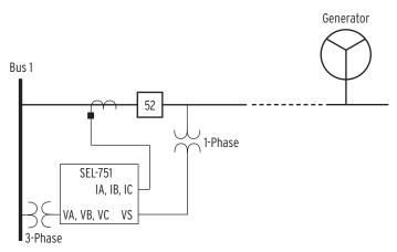
Figure 4.86 Reclose Blocking for Islanded Generator
