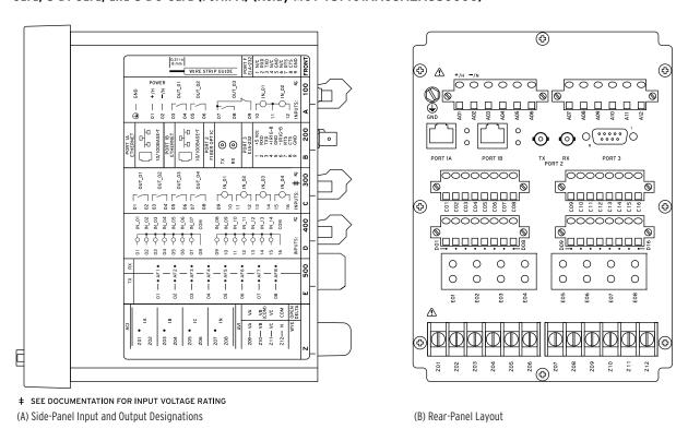
Figure 2.12 Dual Copper Ethernet, 4 DI/4 DO Card, 14 DI Card, 8 AFDI With Arc-Flash Detector Inputs, 4 ACI/3 AVI Card With 5 A Phase, 200 mA Neutral, and Three-Phase AC Voltage Inputs (300 Vac) (Relay MOT 7515S1A1A4A77870671)
