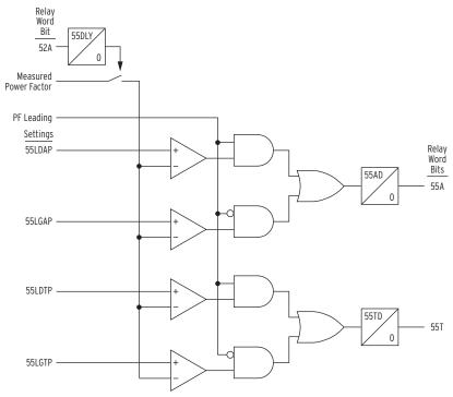
Figure 4.72 Power Factor Elements Logic
