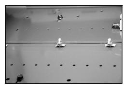
Figure 2.41 Clear-Jacketed Fiber Sensor Mounting Example
