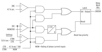
Figure 4.22 Logic for Relay Word bit GNDSW
