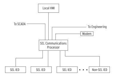
Figure C.1 SEL Communications Processor Star Integration Network
