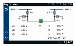
Figure 9.22 Tie Breaker Bay Control Single-Line Diagram
