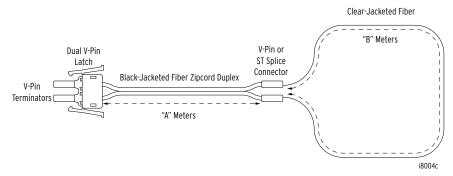
Total loop length =  $2 \cdot A + B$  (allowed range 3 to 70 meters) Range for A: 1 to 30 meters Range for B: 1 to 50 meters
