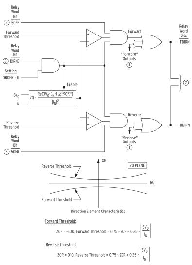
For setting ORDER = U, settings Z0F and Z0R are set internally, as shown above, and hidden. Note:  $1 \angle -90^\circ$  = One Ohm at  $-90^\circ$  Angle
