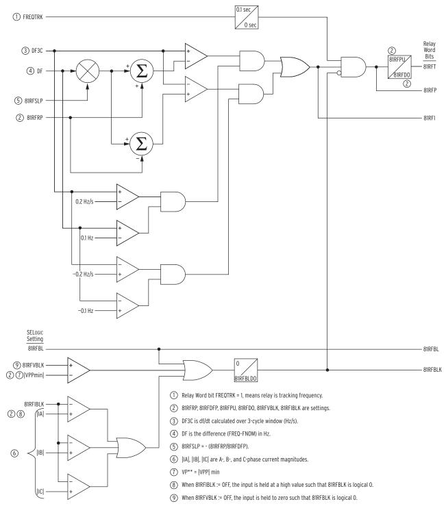
Figure 4.78 81RF Fast Rate-of-Change-of-Frequency Logic
