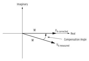
Figure I.3 Correction of Measured Phase Angle
