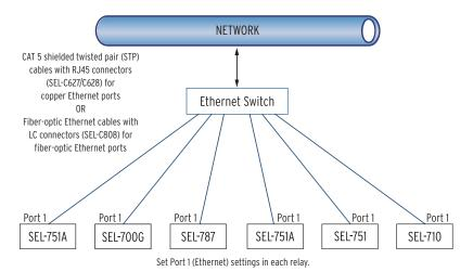
Figure 7.1 Simple Ethernet Network Configuration
