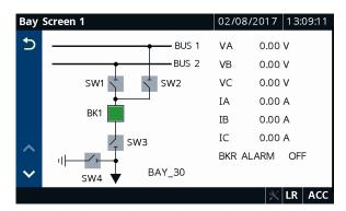
Figure 9.23 Bus 1 and Bus 2 Bay Control Single-Line Diagram
