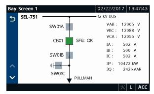
Figure 9.3 Bay Screens Application Display With a Single-Line Diagram
