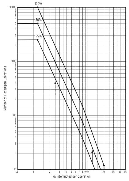
Figure 5.24 Breaker Monitor Accumulates 50 Percent Wear
