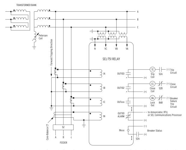
A core-balance current transformer is often referred to as a zero-sequence, ground fault, or window current transformer.
