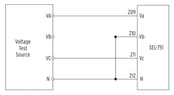
Figure 11.6 Delta Voltage Source Connections
