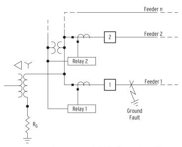
Figure 4.46 Low-Impedance Grounded Distribution System With a Ground Fault on Feeder 1
