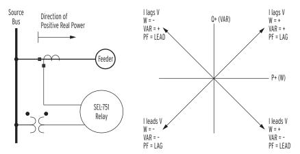
Figure 5.1 Complex Power Measurement Conventions
