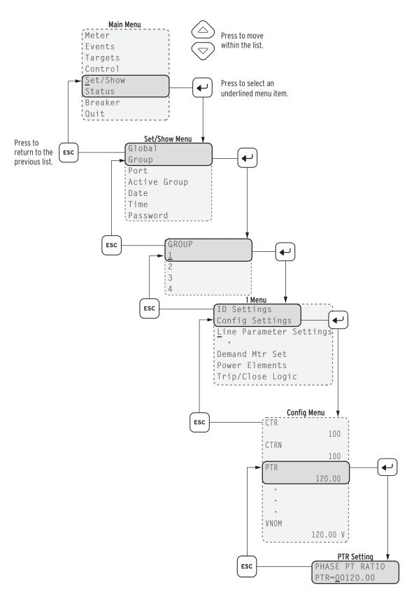
Figure 6.1 Front-Panel Setting Entry Example
