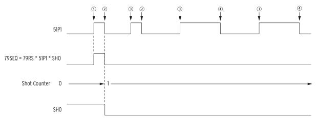
① Fault occurs beyond line recloser; ② fault cleared by line recloser fast curve; ③ line recloser recloses into fault; 4 fault cleared by line recloser slow curve.
