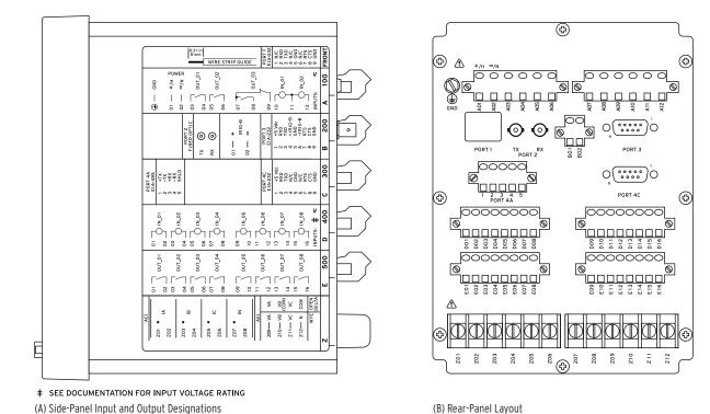
Figure 2.11 No Ethernet, EIA-232 Serial Communications, EIA-232/EIA-485 Communications Card, 8 DI Card, and 8 DO Card (Form A) (Relay MOT 751401AA03A2A850000)
