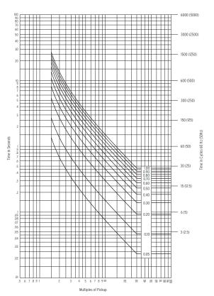
Figure 4.16 IEC Class B Curve (Very Inverse): C2
