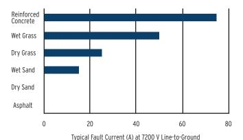
Figure 4.55 High-Impedance Fault Current Levels Depend on Ground Surface Type
