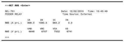
Figure 5.9 METER RMS Command Response
