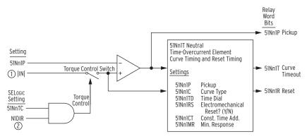
Controls the Torque Control Switch
