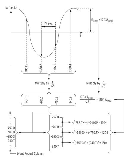
Figure 10.4 Derivation of Event Report Current Values and RMS Current Values From Sampled Current Waveform
