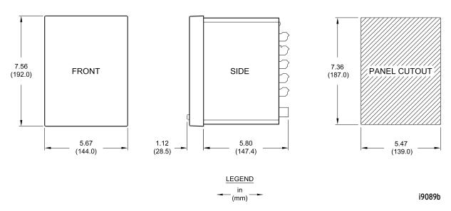
Figure 2.1 Relay Panel-Mount Dimensions
