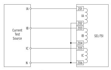
Figure 11.4 Current Source Connections
