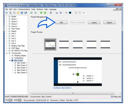
Figure 9.13 Open Single-Line Diagram in Bay Screen Builder
