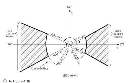
Figure 4.54 Load-Encroachment Logic
