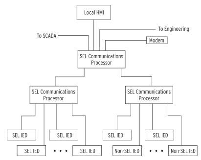
Figure C.2 Multitiered SEL Communications Processor Architecture
