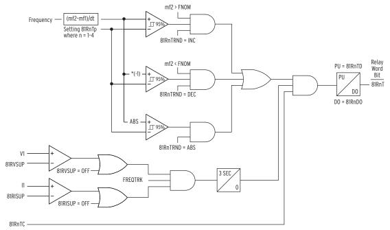
Figure 4.76 81R Frequency Rate-of-Change Scheme Logic
