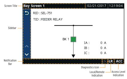
Figure 8.28 Touchscreen Display Components and Indicators
