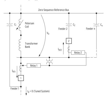
Figure 4.52 Zero-Sequence Impedance Network for Ground Fault on Feeder 1
