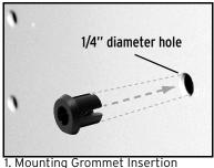
. Mounting Grommet Insertion (1/4" diameter hole)
