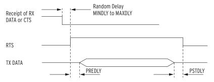
Figure D.2 Message Transmission Timing
