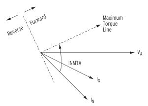
Figure 4.43 Current-Polarized Directional Element Characteristic When INMTA  $\neq$  0.00
