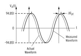
Figure I.2 Waveform at Relay Terminals May Have a Phase Shift
