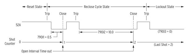
Figure 4.85 Reclosing Sequence From Reset to Lockout With Example Settings
