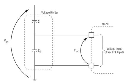
Figure 4.1 Low-Energy Analog Voltage Sensor (Capacitive Voltage Divider)
