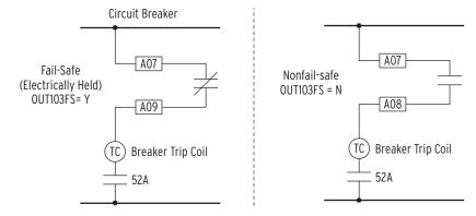
Figure 2.19 OUT103 Contact Fail-Safe and Nonfail-Safe Options
