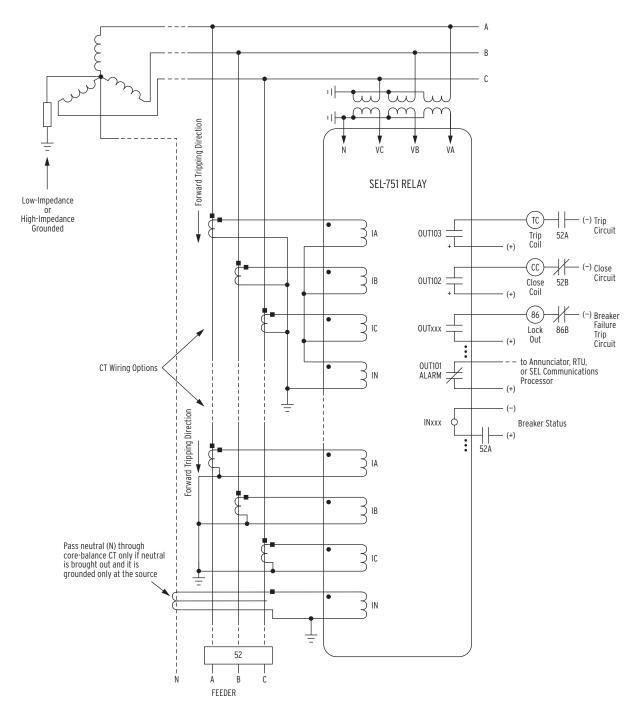
A core-balance current transformer is often referred to as a zero-sequence, ground fault, or window current transformer. The lower CT wiring option (with the core-balance current transformer) is the preferred option (greater sensitivity; no false residual currents due to CT saturation, etc.).
