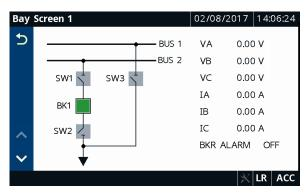
Figure 9.21 Main Bus and Transfer Bus Bay Control Single-Line Diagram
