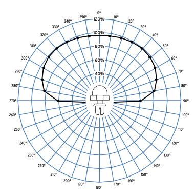
Figure 2.39 Point-Sensor Directivity (Left to Right, Above the Mounting Plane)
