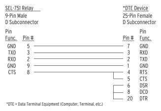
Figure 7.11 SEL Cable C227A-SEL-751 to DTE Device
