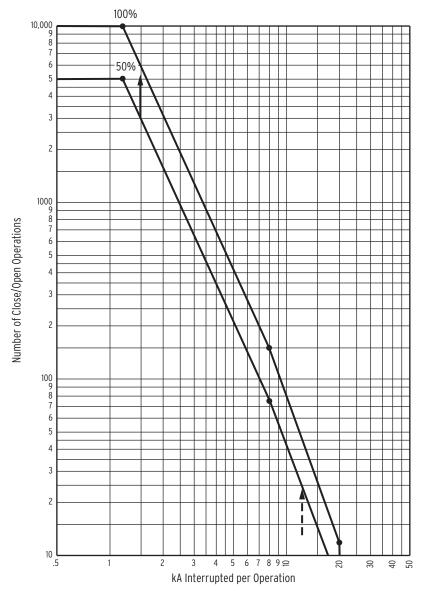
Figure 5.25 Breaker Monitor Accumulates 100 Percent Wear
