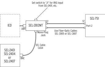
You cannot use **B01-B02** input or Port 3 input if you use Port 2 for IRIG-B input. Set Global setting IRIG TIME SOURCE to TIME\_SRC := IRIG2.
