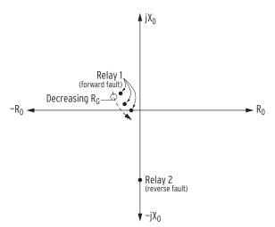
Figure 4.50 Zero-Sequence Impedance Plots for Ground Fault on Low-Impedance Grounded Distribution System
