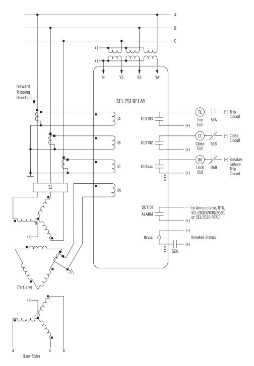
Voltages are necessary for voltage elements, synchronism-check elements, voltage-polarized directional elements, fault location, and metering (e.g., voltage, KW, KVAR). INxxx and OUTxxx indicate user-configurable optional digital inputs and outputs.
