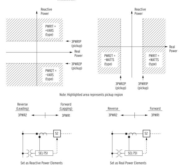
Figure 4.71 Power Elements Operation in the Real/Reactive Power Plane
