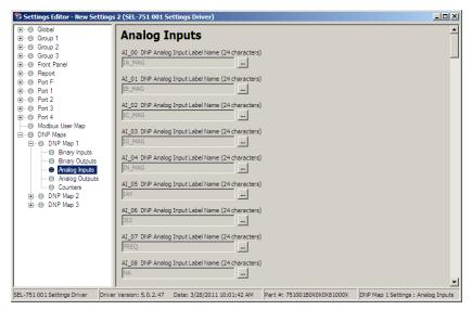
Figure D.6 Analog Input Map Entry in ACSELERATOR QuickSet Software
