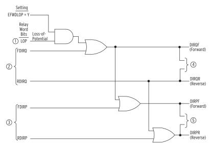
① From Figure 4.73; ② from Figure 4.37; ③ from Figure 4.38; ④ to Figure 4.40; ⑤ to Figure 4.41.
