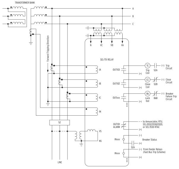
Voltage Channel VS does not need to be connected. Here, it is shown connected for use in voltage and synchronism-check elements and voltage metering. See Figure 2.21 (d and e) on for synchronism-check VS connection (VSCONN := VS) and broken-delta VS connection (VSCONN := 3VO).
