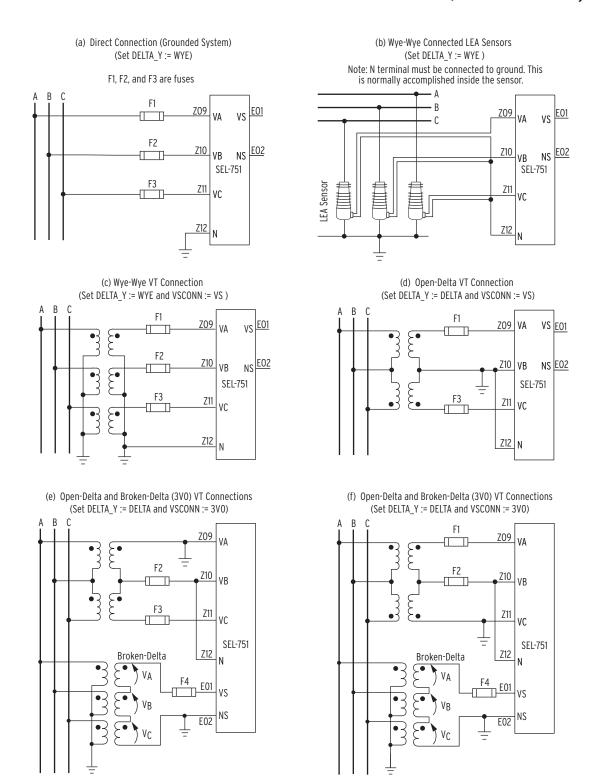
Figure (b) shows LEA inputs, which support only wye-wye connections. Refer to Under- and Overvoltage Functions on page 4.97 and LEA Ratio and Angle Correction Factors (Global Settings) on page 4.8 for the LEA settings and ratio correction factor calculations.
