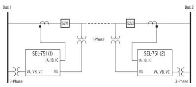
Figure 4.83 SEL-751 Relays Installed at Both Ends of a Transmission Line in a High-Speed Reclose Scheme
