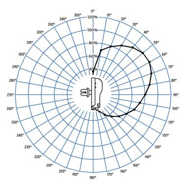
Figure 2.38 Point-Sensor Directivity (Front to Back, Above the Mounting Plane)
