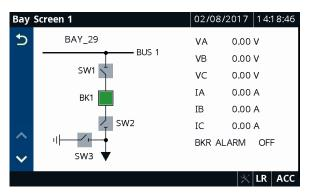
Figure 9.24 Feeder Bay Control Single-Line Diagram
