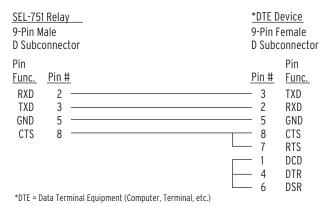
Figure 7.10 SEL Cable C234A-SEL-751 to DTE Device
