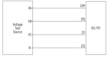
Figure 11.5 Wye Voltage Source Connections
