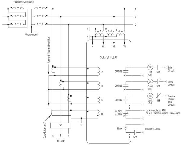
A core-balance current transformer is often referred to as a zero-sequence, ground fault, or window current transformer. Directional control for an ungrounded system is selected with setting ORDER := U (see Table 4.19-Table 4.21). Nondirectional sensitive earth fault (SEF) protection is also available.
