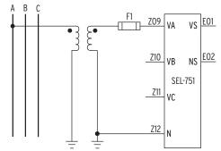
Figure 2.20 Single-Phase Voltage Connections
