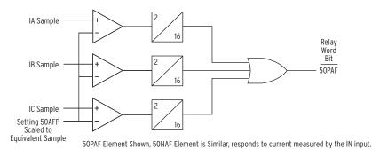
Figure 4.102 Arc-Flash Instantaneous Overcurrent Element Logic
