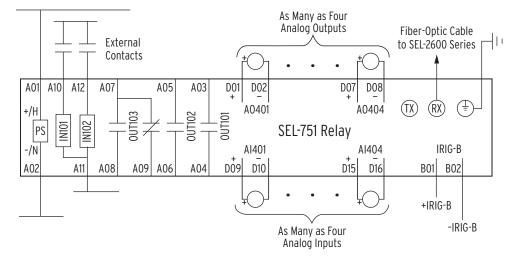
Figure 2.15 Control I/O Connections-4 AI/4 AO Option in Slot D and Fiber-Optic Port in Slot B
