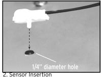
. Sensor insertion (1/4" diameter hole)
