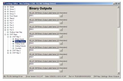
Figure D.11 Binary Output Map Entry in ACSELERATOR QuickSet Software
