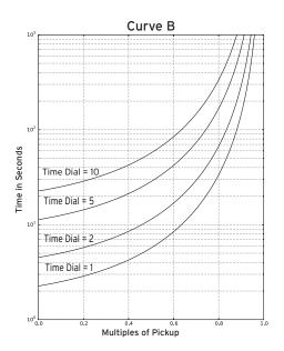
Figure 4.64 Inverse Time-Undervoltage Element Curves
