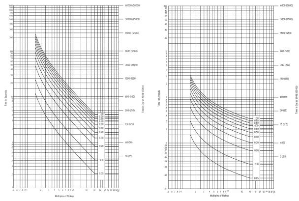
Figure 4.18 IEC Long-Time Inverse Curve: C4
