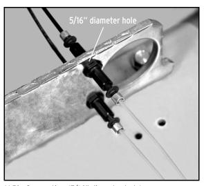
V-Pin Connection (5/16" diameter hole)
