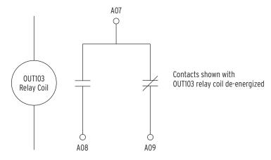
Figure 2.18 Output OUT103 Relay Output Contact Configuration
