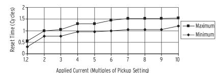
Figure 4.4 Instantaneous Overcurrent Element Reset Time Curve
