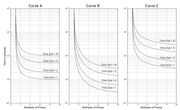
Figure 4.66 Inverse Time-Overvoltage Element Curves
