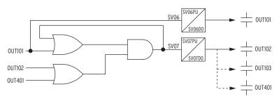
Figure 4.97 Example Use of SELogic Variables/Timers
