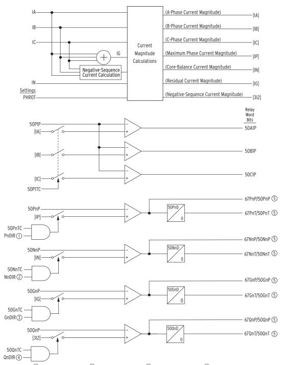
① To Figure 4.41; ② From Figure 4.35; ③ From Figure 4.34; ④ From Figure 4.40; ⑤ Residual Current Magnitude IIGI is the calculated residual current. Not shown in the figure, Relay Word bit ORED50T is asserted if any of the 50PnT, 67PnT, 50NnT, 67NnT, 50GnT, 67GnT, 50QnT or 67QnT Relay Word bits are asserted (n = 1 to 4).
