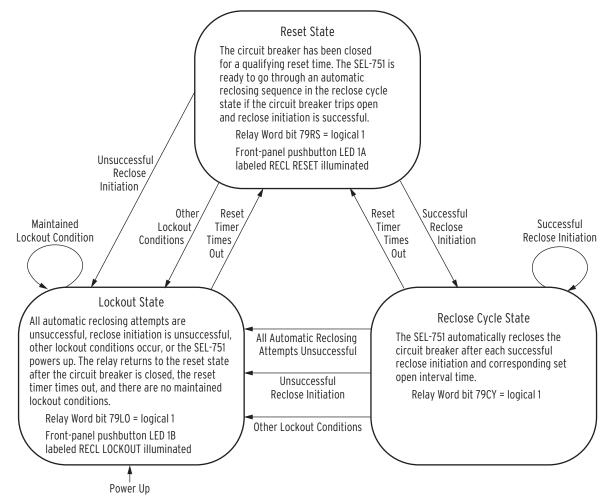
Figure 4.84 Reclosing Relay States and General Operation
