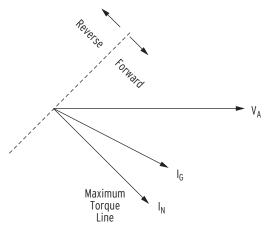
Figure 4.42 Traditional Channel IN Current-Polarized Directional Element
