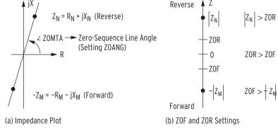
Figure 4.45 Zero-Sequence Impedance Plot for Solidly-Grounded, Mostly Inductive System
