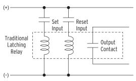
Figure 4.93 Schematic Diagram of a Traditional Latching Device
