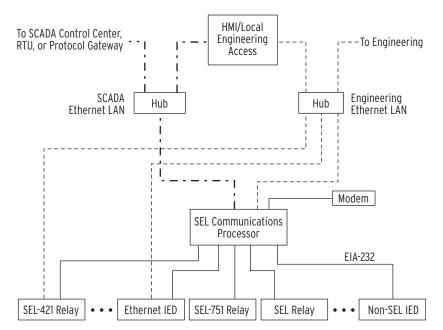
Figure C.3 **Enhancing Multidrop Networks With SEL Communications Processors**
