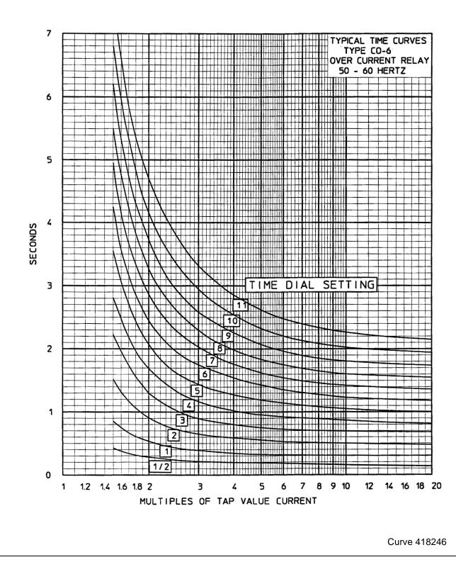
Figure 15: Typical Time Curve of the Type CO-6 Relay
