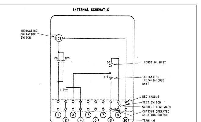
Figure 9: Internal Schematic of the Single Trip Relay With ITT Contacts Wired to Two Separate Terminals
