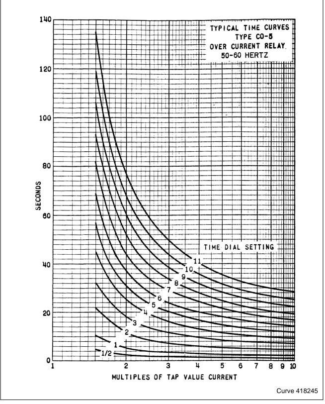
Figure 14: Typical Time Curve of the Type CO-5 Relay
