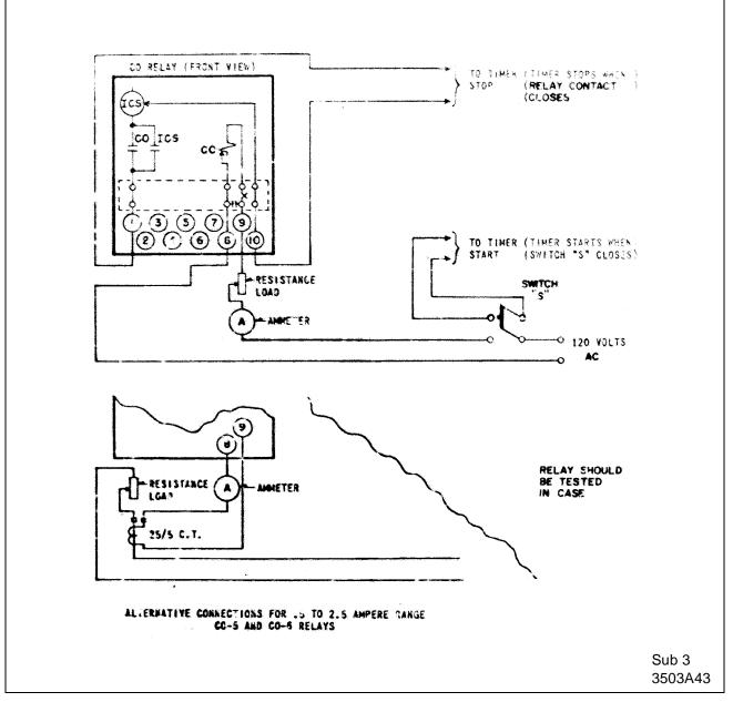
Figure 3: Diagram of Test Connections for Circuit Closing Type CO Relay
