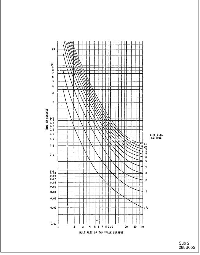
Figure 19: Typical Time Curve of the Type CO-11 Relay
