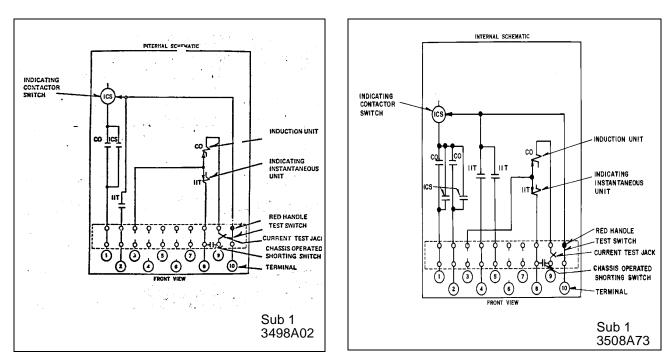
Figure 7: Internal Schematic of the Single Trip Relay With IIT
