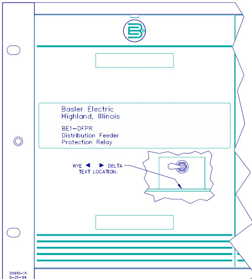
Figure 2-6. Wye/Delta Switch Location In Magnetism Module, Horizontal Mount
