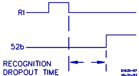
Figure 3-4. Recognition Dropout Timing
