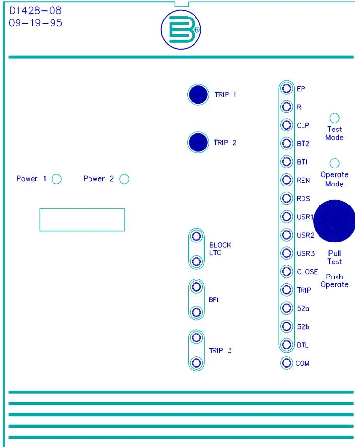
Figure 2-4. Contact Sense Module, Front Panel
