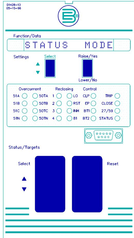
Figure 2-3. Control Module, Front Panel, Horizontal Mount
